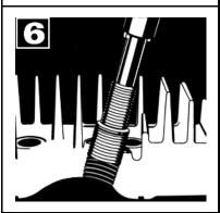
**6.** Note: <u>Tapered Seat inserts</u> these inserts are silver plated and require sealer p/n 6020 on the outside of the insert.
