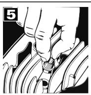
Make sure the hole is clean and dry. Lubricate the driver tool with Time-Sert driver oil. Screw the insert onto the prepared hole.
