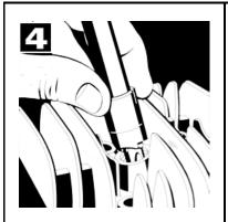
4. Using the wrench provided rotate the seat cutter. After a few turns lift the seat cutter to inspect the seat. Repeat operation until the seat is completely cleaned up. Remove the step tap from the hole. **Bad seat Good seat**
