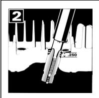
Using the wrench provided place wrench over tap and tap new threads. Continue to tap through until the cutting edges are approximately 1/4 inch below surface.
