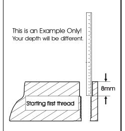
1. Using the metal rule measure from the top of the surface to the First starting thread.
